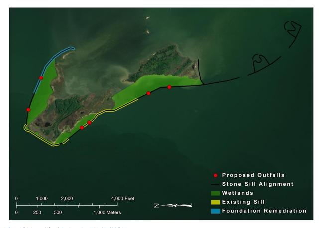
Figure 2 Barren Island Restoration Total Build Out
